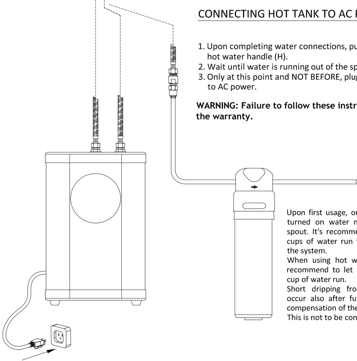
Upon first usage, once the hot tank is turned on water may drip from the spout. It's recommended to let 2 1/4 cups of water run to clear and prime the system.
